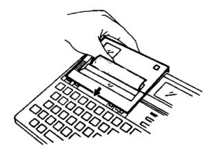
\* To take out the paper from the printer, pull the paper straight out from the paper case side or from the paper cutter side.
