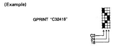
The 8-dot patterns specified by the hexadecimal number pairs are arranged to draw the picture.
